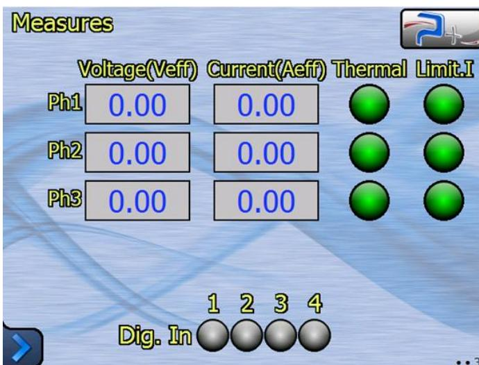
On the measurements screen, fields return the instantaneous values of voltage and current.
