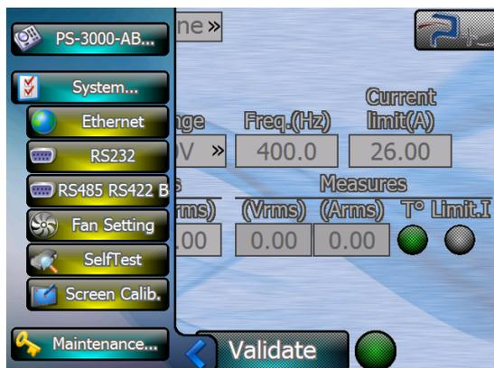
Other screens are to set up communications links or for the management of variable speed fans.
