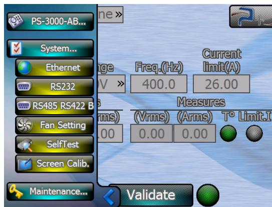
Other screens are to set up communications links or for the management of variable speed fans.
