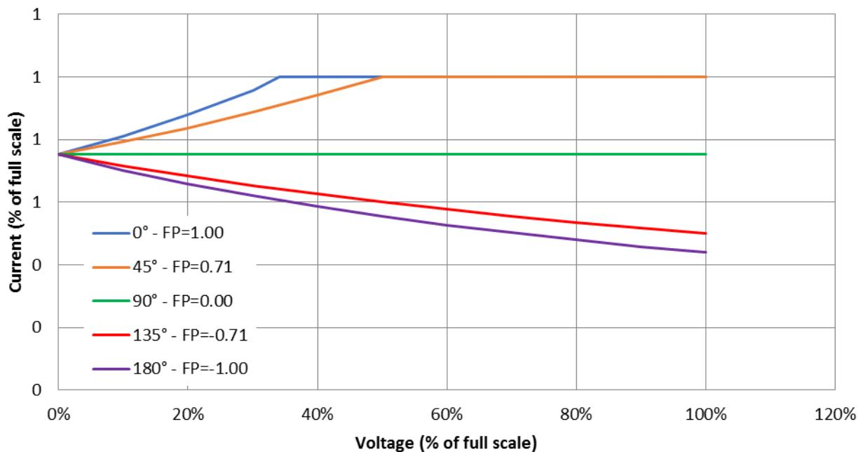
**Blue:** phase shift between the voltage and the current is zero (in phase). FP power factor = +1 (generation on resistive load).
