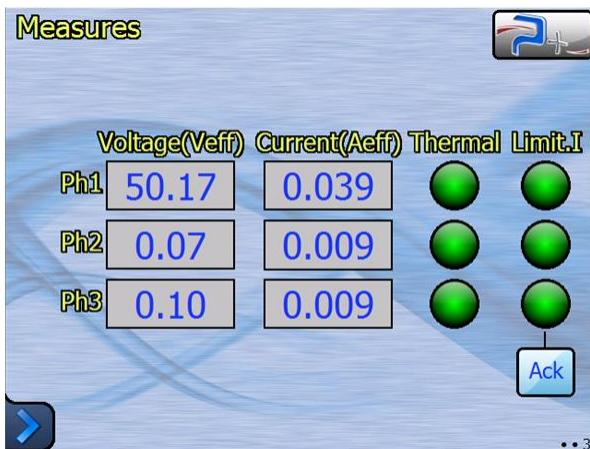
Measurement screen displays voltage and current measurements and overheating or overcurrent information.
