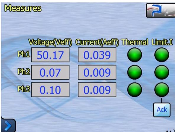
Measurement screen displays voltage and current measurements and overheating or overcurrent information.
